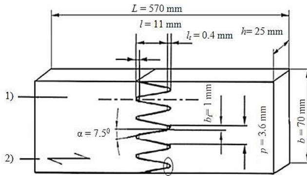
**Figure 2.** Linear and angle parameters of the finger joint:  $l$  – length of fingers;  $p$  – step of fingers;  $b_f$  – width of the finger;  $l_i$  – tolerance of the finger joints end;  $\alpha$  – side angle of the finger joint;  $L$  – length of testing piece;  $h$  – thickness of the testing piece;  $b$  – width of the piece; 1) – way of symmetry of the finger joint; 2) – fibre direction of the testing piece (DIN68140EErI ND, 1981).
