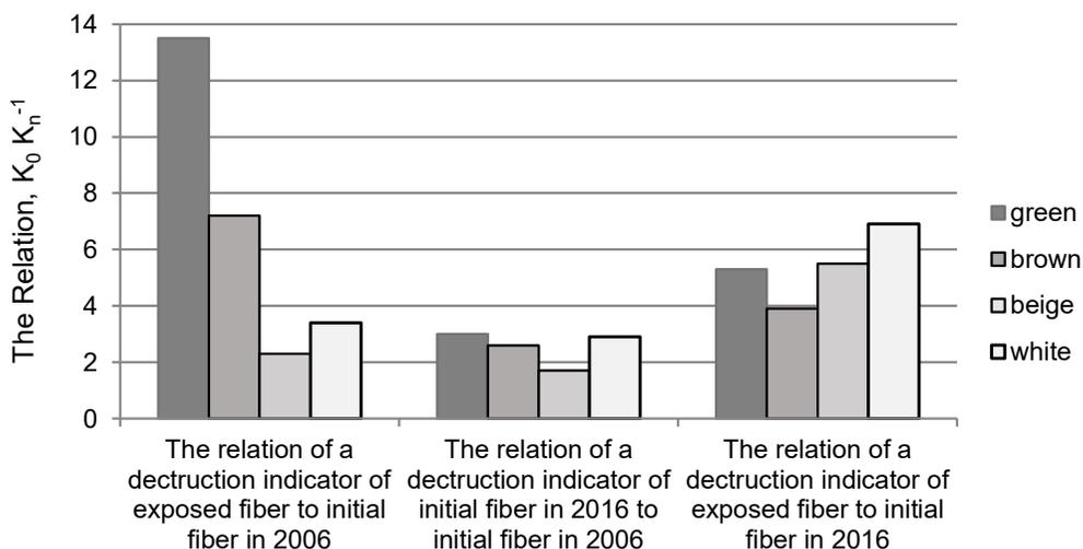
**Figure 2.** Changes in the cotton fibers' destruction indicator in various storage conditions;  $K_0$  – the initial fiber destruction indicator (start of storage period);  $K_n$  – the exposed fiber destruction indicator.
