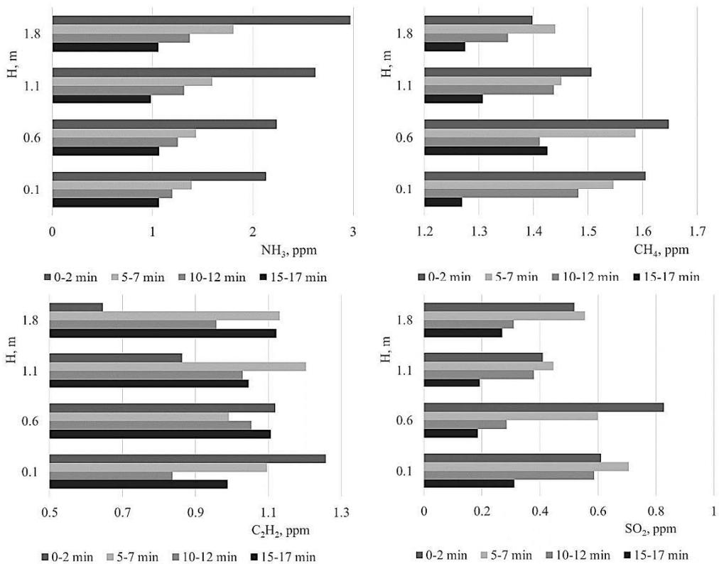
**Figure 4.** Variation of main unregulated emissions ( $\text{NH}_3$ ,  $\text{CH}_4$ ,  $\text{C}_2\text{H}_2$  and  $\text{SO}_2$ ) for diesel engine (Volvo V70 2.5TDI).
