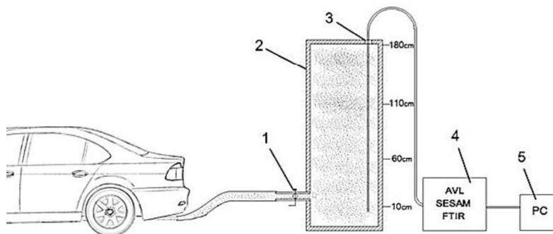
**Figure 1.** Schematic diagram of experimental setup: 1 – inlet valve; 2 – gas storage tank; 3 – probe loading aperture; 4 – multicomponent exhaust gas measurement system AVL SESAM FTIR; 5 – data recording PC.
