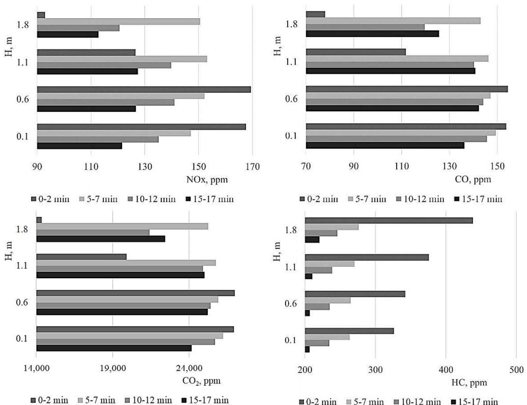
**Figure 2.** Variation of main regulated emissions (NO<sub>x</sub>, CO, CO<sub>2</sub> and HC) for diesel engine (Volvo V70 2.5TDI).
