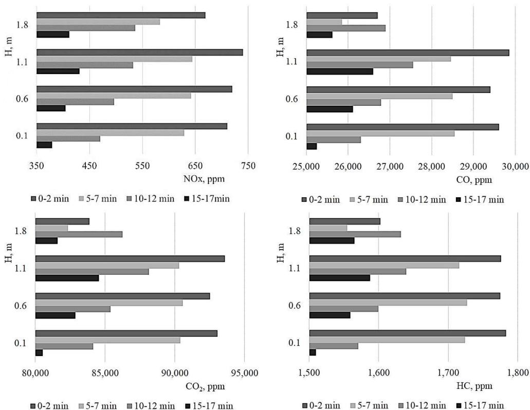
**Figure 3.** Variation of main regulated emissions (NO<sub>x</sub>, CO, CO<sub>2</sub> and HC) for gasoline engine (Audi A6 2.6).
