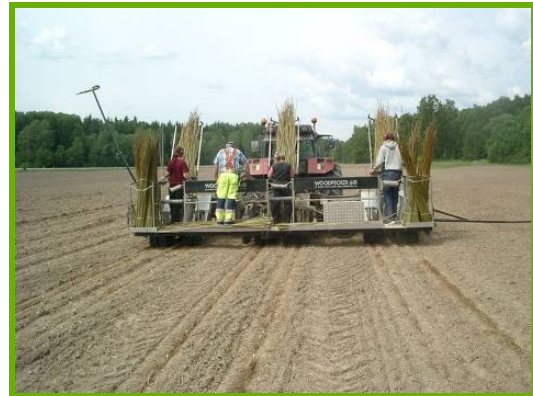
Picture 11. For SRP planting different types of machinery can be used. The time and work load required for one hectare of short cuttings planting (A) is much larger than for long rod step-planting (B). [Photos by: T. Tilger, EAU; N.-E. Nordh, SLU respectively]
