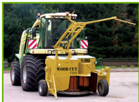
Picture 19. Chipping with CLAAS HS-2 (left) and KRONE Woodcut header (right). [Photo by: CLAAS, KRONE]
