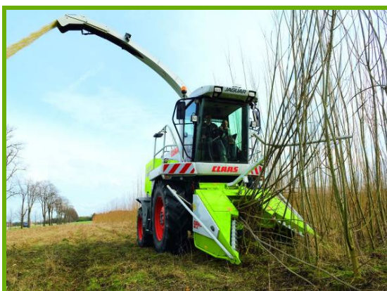
Picture 19. Chipping with CLAAS HS-2 (left) and KRONE Woodcut header (right). [Photo by: CLAAS, KRONE]
