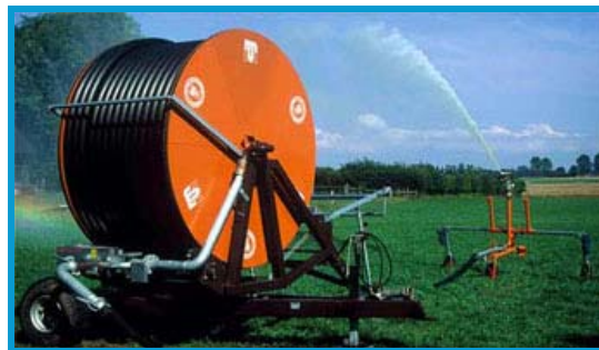
Picture 40. Sprinklers [Photo by: RMV AB]
