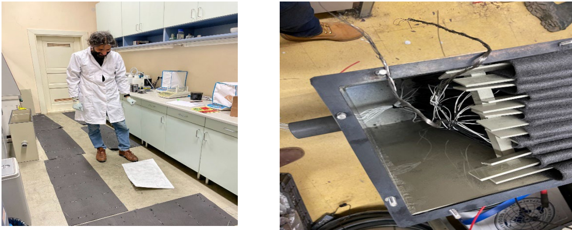
Figure 4. Assembling the reactor, anodes and cathodes, wiring before and after installation.
