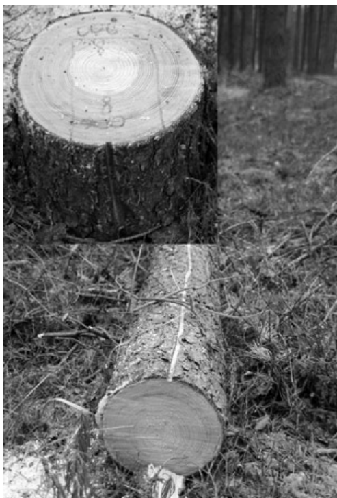
Figure 3. A felled sample tree in the forest with the marked eastern side and a cut sample block (annual shoot) with the contours of the further sample body (original photo).
