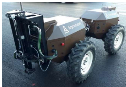
Figure 2. Articulated steering UGV platform prototype with soil sampling mechanism.
