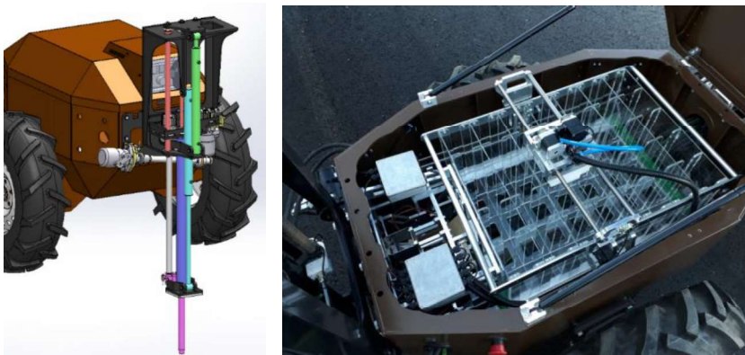
Figure 3. Soil sampling mechanism CAD-model (left) and sample storage system from the prototype.
