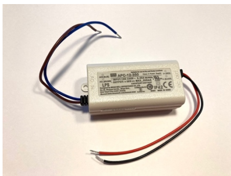
Figure 16. Constant current power supply for 3-10 LEDs.
