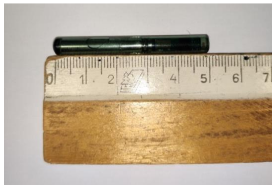
Figure 2. Example of the temperature sensor implant that was used for all calves in this study (Author: Tarmo Niine, EMÜ)
