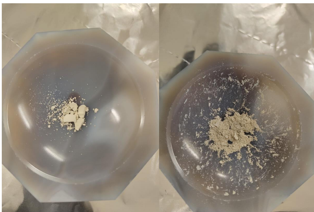
Figure 3.12. ZnO nanoparticles before (left) and after (right) crushing.
