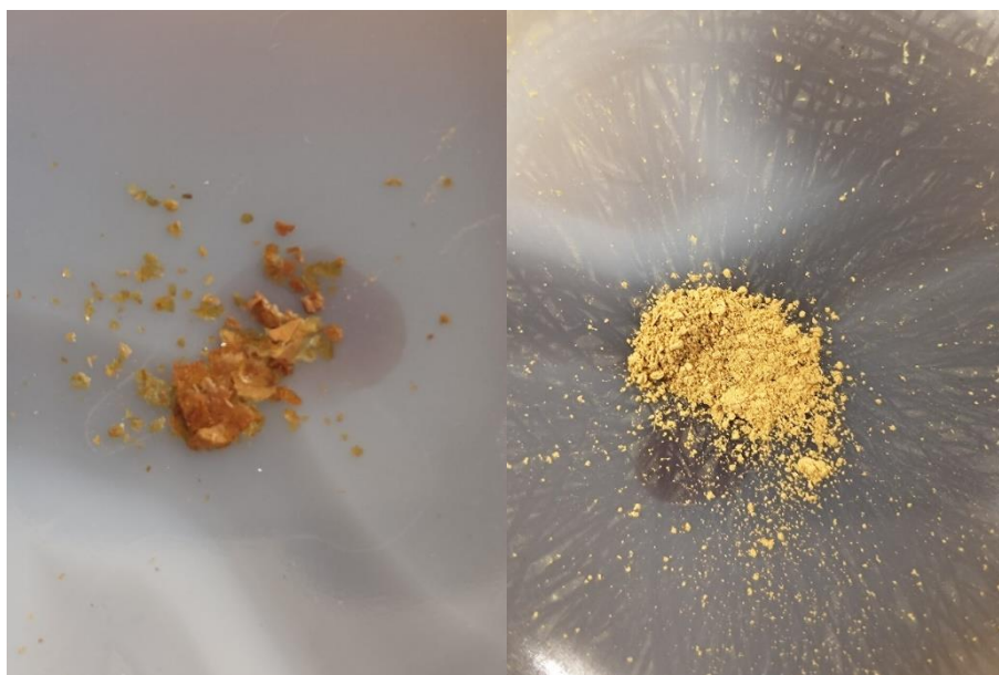
Figure 3.10. Al 2 O 3 nanoparticles before (left) and after (right) crushing.
