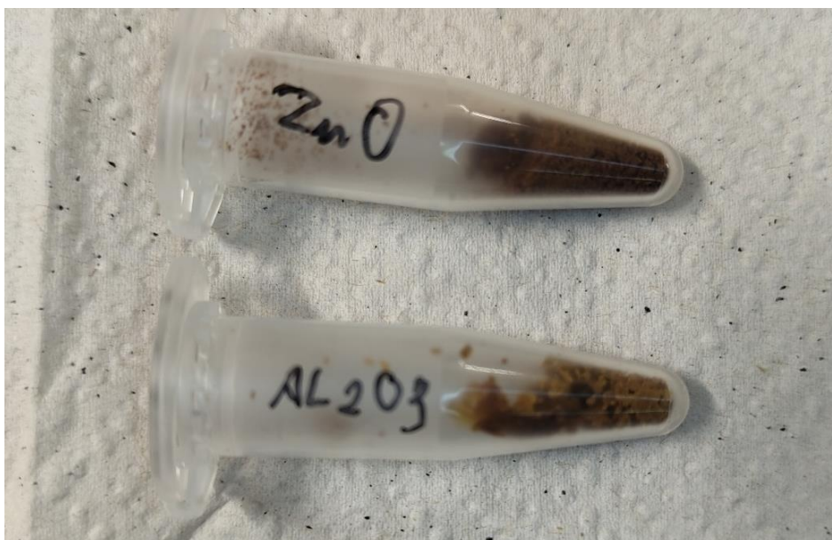
Figure 3.3. ZnO nanoparticles (top) and Al 2 O 3 nanoparticles (bottom) after crushing.
