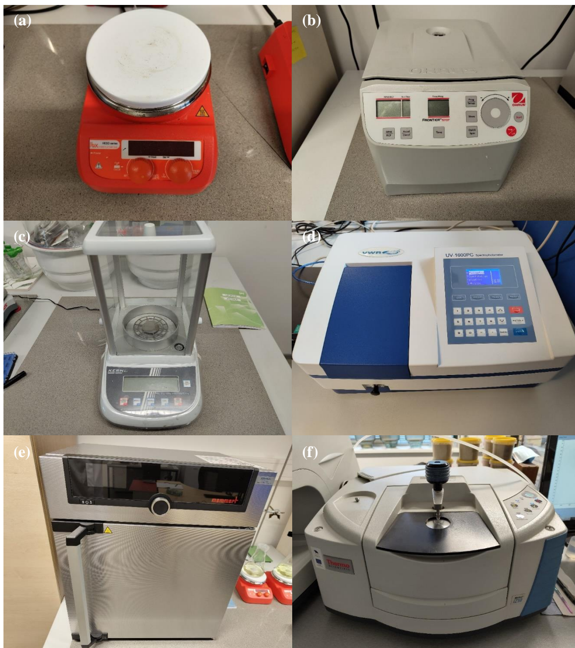
Figure 2.1. Used laboratory equipment LBX H03D (a), Ohaus Frontier FC5707 (b), Kern ALJ 200 (c), VWR UV-1600PC (d), Memmert MMT-UN30 (e), ThermoFisher Nicolet iS10 (f).
