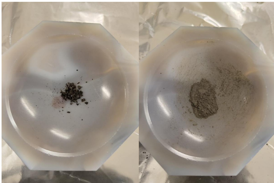
Figure 3.15. ZnO nanoparticles before (left) and after (right) crushing.
