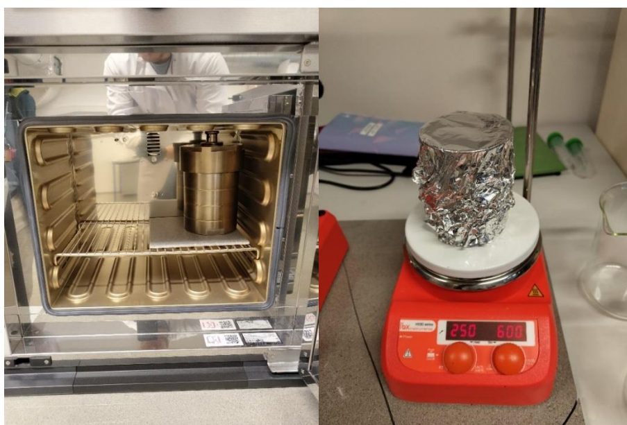
Figure 3.4. Aluminium solution in the oven (left) and zinc solution on the heating plate (right).
