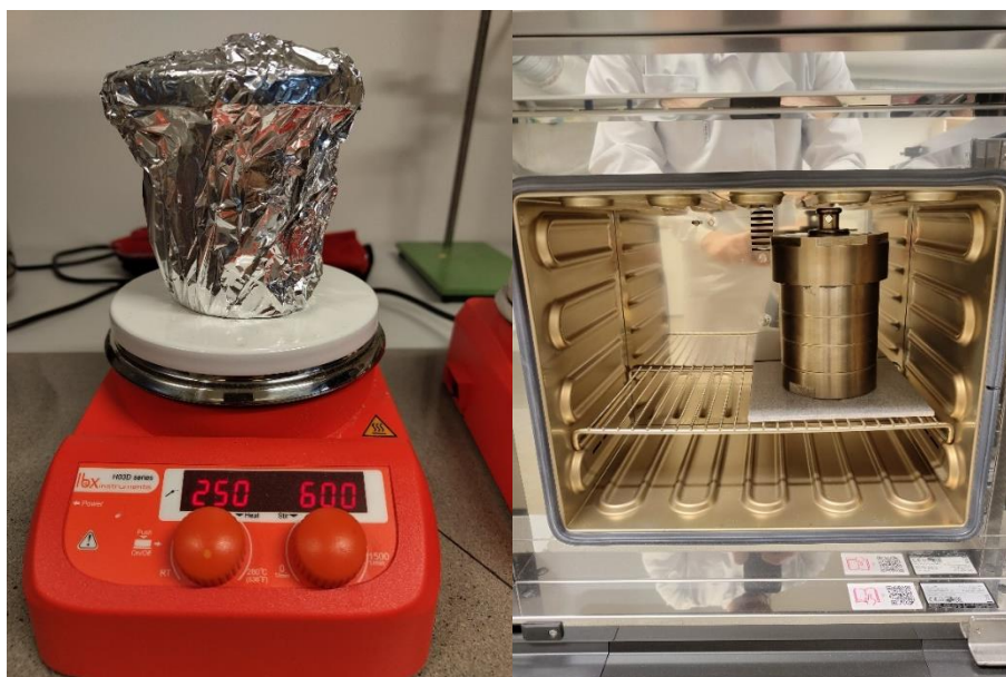
Figure 3.6. Aluminium solution on the heating plate (left) and zinc solution in the oven (right).
