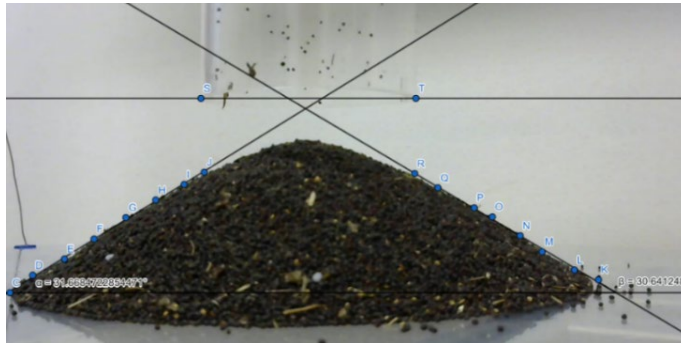
Figure 6. Measuring the angle of repose on the real system.
