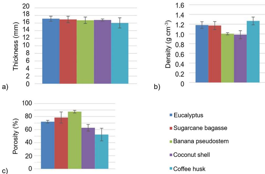
**Figure 3.** Physical properties of the lignocellulosic panels: a) Thickness (mm); b) Density (g cm<sup>-3</sup>); c) Porosity (%) of Eucalyptus, sugarcane bagasse, banana pseudostem, coconut shell and coffee husk.
