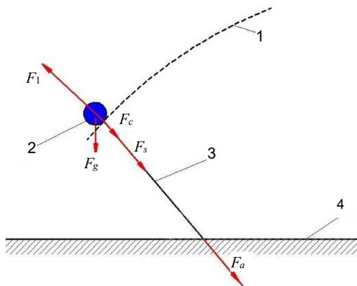
**Figure 3.** Those forces which are applied to a blueberry plant by the harvesting machinery flexible picking teeth: 1 – the picking reel's teeth; 2 – the berry on the blueberry plant; 3 – the blueberry stem; 4 – the field surface.
