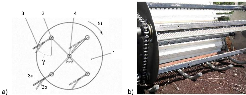
**Figure 2.** The blueberry harvester's picking reel: a) the principal schematic; b) prototype, with 1 – picking reel, 2 – picking rake, 3 – rake tooth, 3a – straight tooth, 3b – bent tooth, and 4 – spindle.
