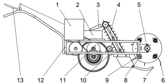
**Figure 1.** The main assemblies and parts of a motoblock-type harvester: 1 – engine; 2 – berry box; 3 – chute; 4 – conveyor; 5 – picking reel; 6 – hook spring-tine; 7 – copying unit; 8 – picking rake; 9 – rake tooth; 10 – wheels; 11 – transmission; 12 – frame; and 13 – steering levers.
