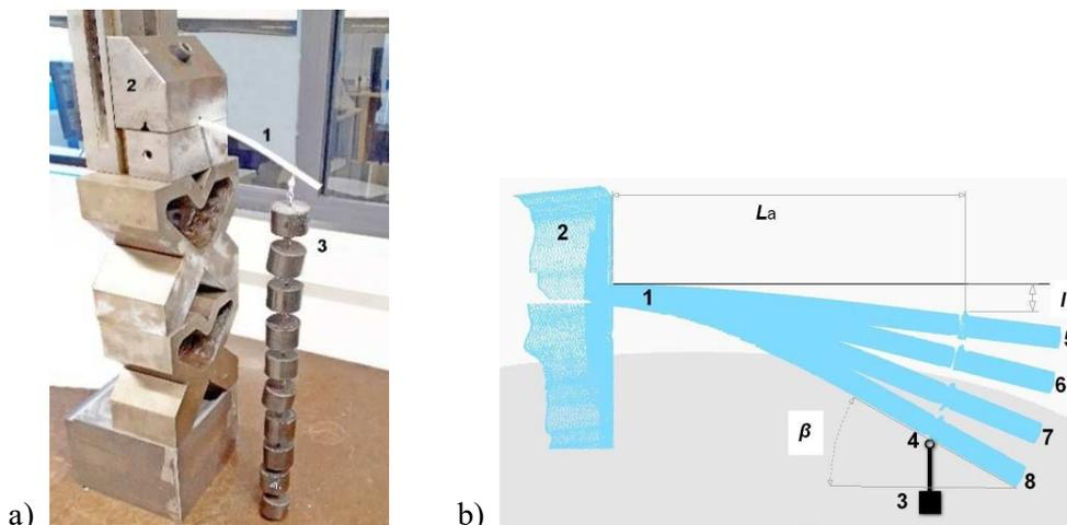
**Figure 6.** Test stand for measuring the tooth’s flexure, a): and a digital model of the tooth’s flexure b): with three weights (position 5), six weights (position 6), nine weights (position 7), and twelve weights (position 8), where  $l$  is the flexure of the cantilever beam and  $L$  is the distance between the cantilever attachment point and the weight attachment.
