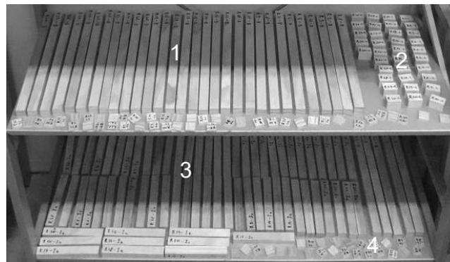
**Figure 1.** Example of radiata pine specimens: 1 – bending strength and modulus of elasticity specimens 2 – moisture content, density and compression strength specimens; 3 – resistance to impact specimens and 4 – swelling specimens.
