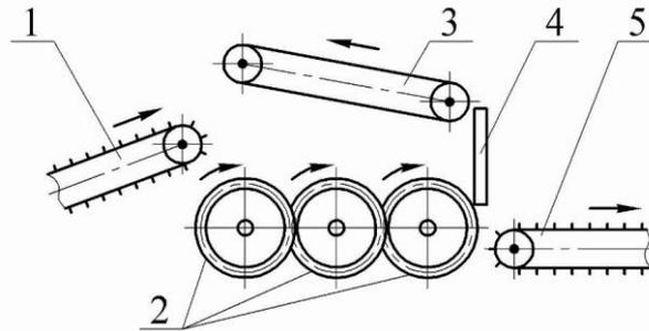
**Figure 1.** Potato heap separator of improved design (side view): 1 – feeding conveyor; 2 – cantilevered spiral springs of cleaning rolls; 3 – rebounding belt conveyor; 4 – protecting apron; 5 – discharge conveyor.
