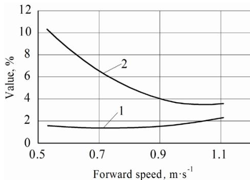
**Figure 6.** Relation between potato tuber loss (1) / damage (2) rates and field pilot unit travel speed (Bulgakov et al., 2017).
