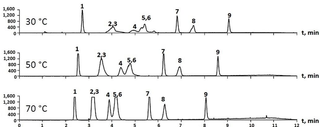
**Figure 2.** UPLC-ELSD chromatograms of several biomass related sugars with column temperature 30, 50 and 70 °C: 1 – levoglucosan; 2 – xylose; 3 – arabinose; 4 – mannose; 5 – glucose; 6 – galactose; 7 – sucrose; 8 – cellobiose; 9 – raffinose.
